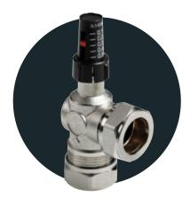
A sudden pressure increase activates the differential pressure control valve, to prevent an excessive drop in the water circulation in the central heating system. The differential pressure control valve also prevents annoying noise and ensures a sufficient flow rate, which prevents the central heating system boiler pump from overloading.
